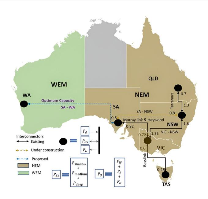
NEM interconnected with WEM, along with interconnectors between different regions of NEM with transmission line forward capacities in GW. The SA–NSW
