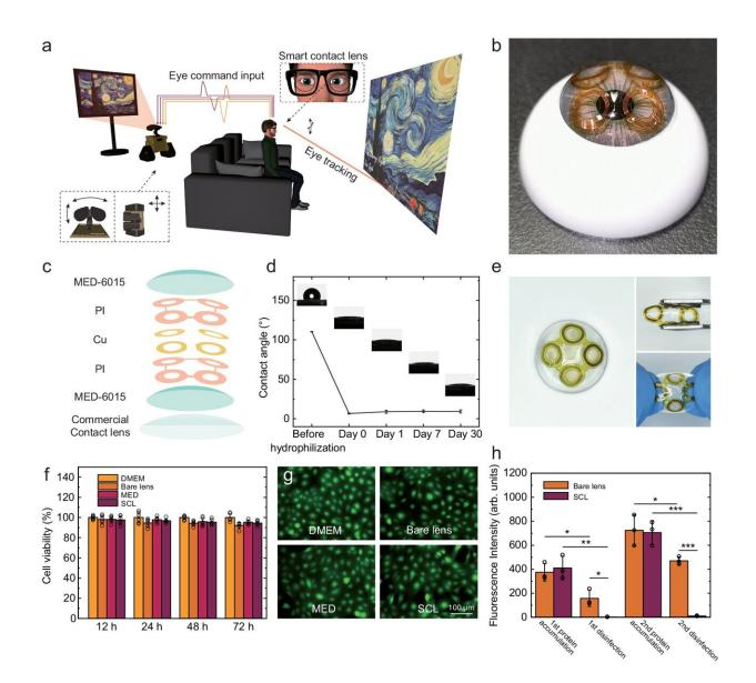
Human-machine interaction by eye-tracking using smart contact lens. b) shows a photograph of the lens. Credit: *Nature Communications* (2024). DOI:
