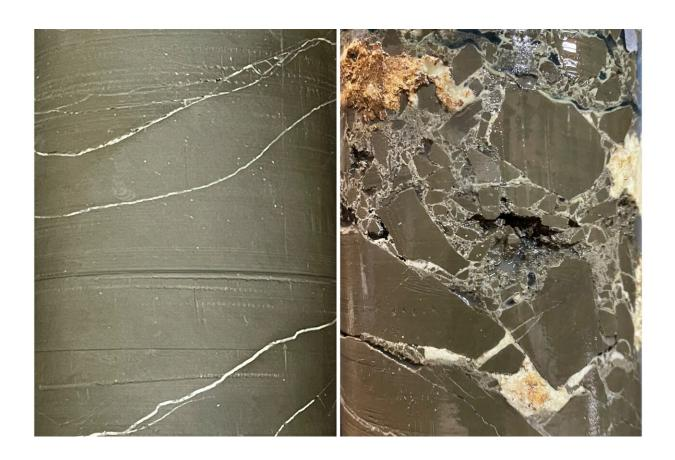
Flow-path fractures in rock sealed by calcite, promoted by the researchers' 'concretion-forming resin'. Credit: Hidekazu Yoshida
