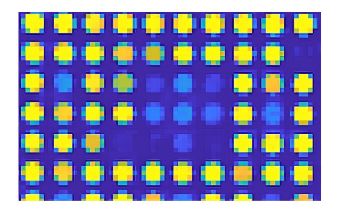
The cross-section image of a fuel rod assembly shows individual rods, like a handful of pencils seen from above. Credit: Riina Virta
