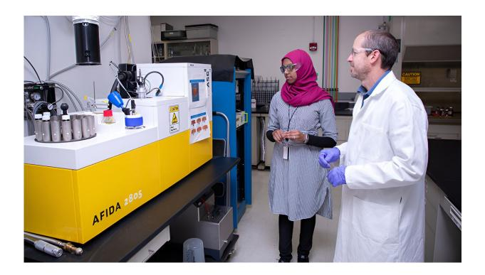
NREL researchers Jon Luecke (right) and Samah Mohamed perform fuel analyses using an Advanced Fuel Ignition Delay Analyzer (AFIDA) in the Fuels Lab. Credit: Joe DelNero, NREL
