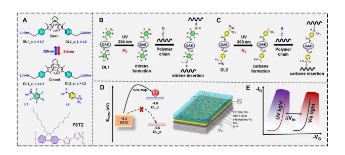
A. F8T2 polymer employed in tandem with the molecular framework of a molecular switch including a photocrosslinker. Credit: POSTECH
