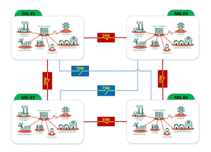
A reconfigurable multi-microgrid system. Credit: *Electric Power Systems Research* (2024). DOI: 10.1016/j.epsr.2024.110285
