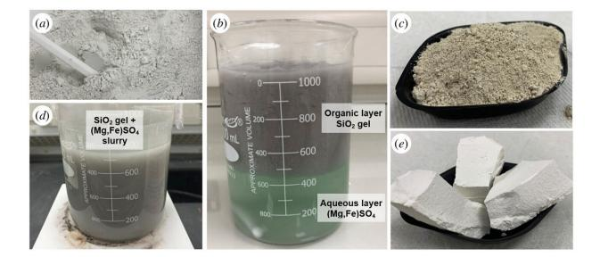
Photographs showing (a) raw as-received olivine, (d) dissolution of the olivine using H2SO4, (b) separation of silica gel from magnesium/iron sulfate using IPA, (c) APS and (e) HMC nesquehonite. Credit: *Royal Society Open Science* (2024). DOI: 10.1098/rsos.231645
