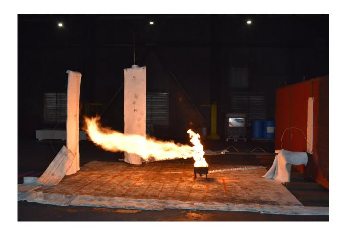
In this image, natural gas is discharged through a two-inch diameter pipe and ignited as part of an SwRI-conducted test to evaluate pressure relief valves. Temperatures and heat fluxes were measured at different standoff distances to provide computer model validation data that can aid future researchers as they investigate a variety of accident scenarios. Credit: Southwest Research Institute
