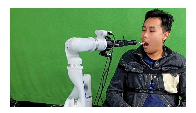
A robotic system developed by Cornell researchers feeds a student participant during a lab demonstration. Credit: Cornell University
