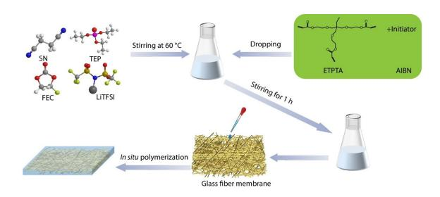
Schematic illustration of the manufacture procedure of the SN-based electrolytes. Credit: *Chinese Journal of Polymer Science* (2023). DOI: 10.1007/s10118-023-2970-y
