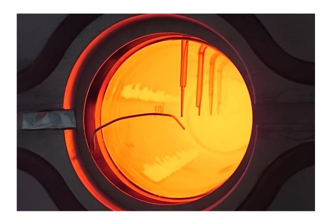
Thermal-trapping device reaching 1050 degrees Celsius. Credit: Device/Casati et al.
