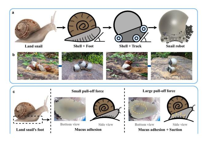
a Morphological evolution from a snail to a snail robot. b Snails outdoors may climb onto another snail's shell for various reasons. Inspired by this, snail robots can also interconnect with each other. c Comparative illustration of snail foot adhesion and snail robot connection mechanism under varying external forces. Credit: *Nature Communications* (2024). DOI: 10.1038/s41467-024-47788-2
