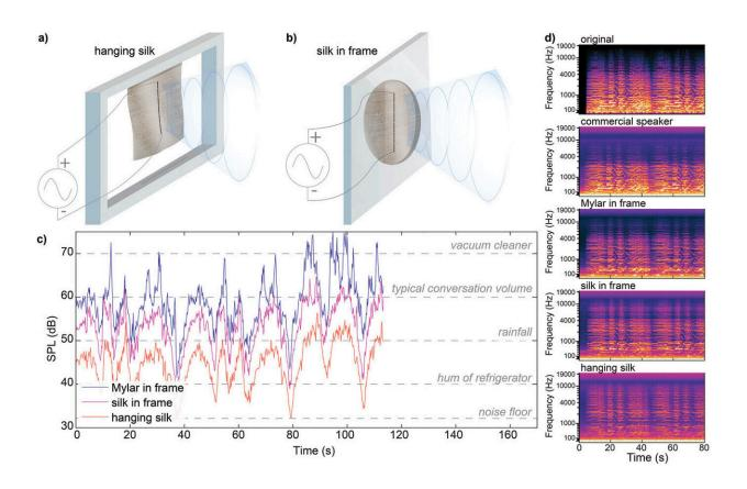
Silk fabric samples a) in a hanging state and b) mounted in a circular frame. Credit: *Advanced Materials* (2024). DOI: 10.1002/adma.202313328
