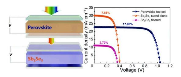
Demonstration of a proof-of-concept tandem solar cell composed of antimony selenide and wide-band-gap perovskite as bottom and top subcell absorption materials. The device achieves a greater than 20% power conversion efficiency by optimizing the transparent electrode of the top cell and the preparation process of the bottom cell. Credit: Energy Materials and Devices, Tsinghua University Press
