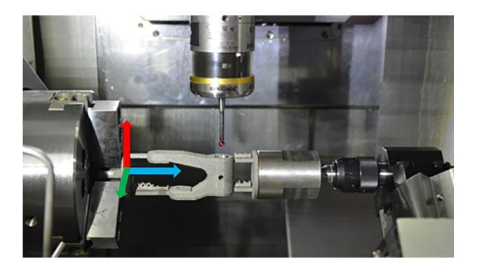
Example of a 3D-printed part mounted in the computer numerical control machine after finishing work; the touch probe is preparing to take automated measurements. Credit: Brandon McConnell, NC State University
