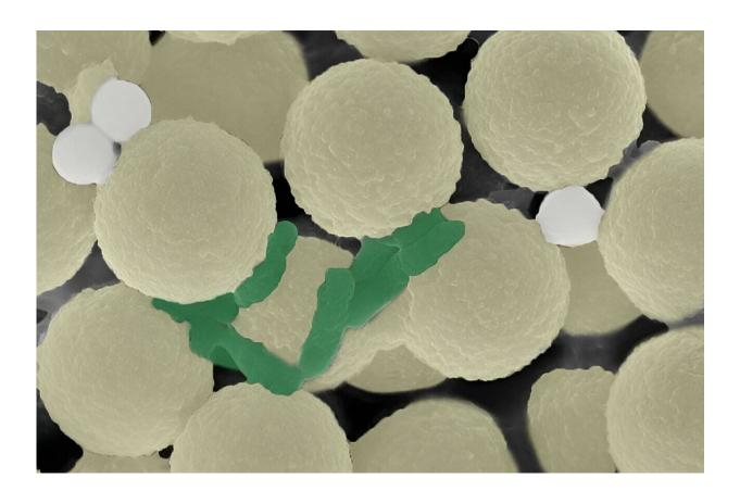
To clean water, researchers have designed swarms of tiny, spherical robots (light yellow) that collect bacteria (green) and small pieces of plastic (gray). Credit: Adapted from ACS Nano 2024, DOI: 10.1021/acsnano.4c02115
