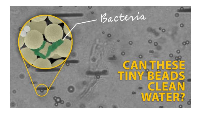
To clean water, researchers have designed swarms of tiny, spherical robots that collect bacteria and small pieces of plastic. Credit: American Chemical Society
