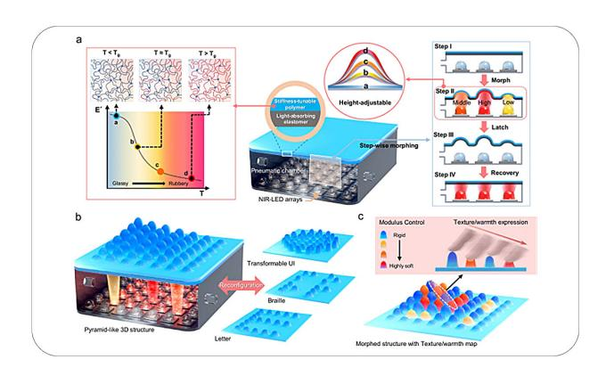
Tactile Display Structure and Operation Principle. Credit: Electronics and Telecommunications Research Institute(ETRI)
