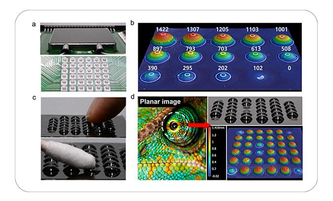
3D Shape and Elasticity Representation by the Tactile Display. Credit: Electronics and Telecommunications Research Institute(ETRI)
