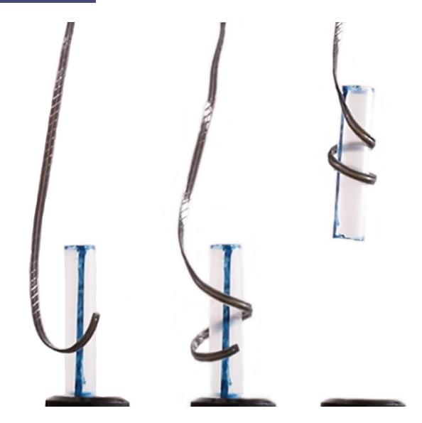
The miniature soft hydraulic actuators can control the deformation and motion of soft robots that are less than a millimeter thick. This photo shows a tendril-like soft robot wrapping around a cylinder and lifting it up. Credit: Jie Yin, NC State University
