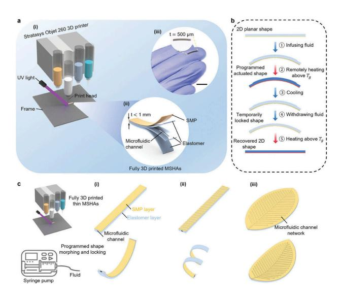
Schematic illustrations of the fully 3D-printed miniature sub-millimeter-thick soft hydraulic actuator (MSHA) integrated with the SME for shape morphing and shape locking. Credit: *Advanced Materials* (2024). DOI:
