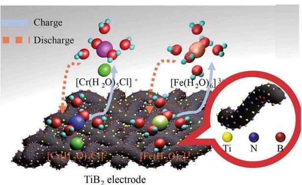
Preparation of N-B doped composite electrode for iron-chromium redox flow battery. Credit: Green Energy and Intelligent Transportation
