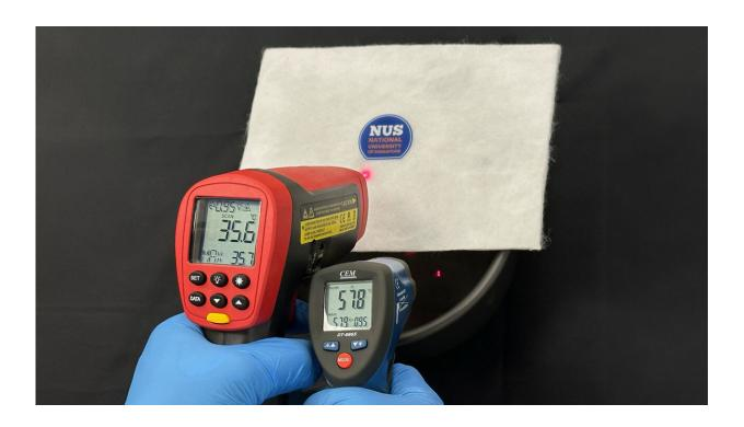
In this demonstration, the white aerogel insulates the area underneath from the surrounding heat, while simultaneously cools the area through radiative cooling, as shown by the lower temperature on the upper surface of the aerogel compared to the temperature of the hot water basin. Credit: National University of Singapore
