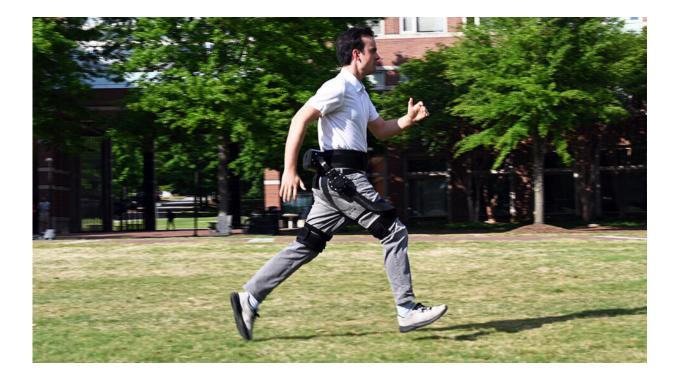
Researchers at North Carolina State University have demonstrated a new method that leverages artificial intelligence and computer simulations to train robotic exoskeletons to autonomously help users save energy while walking, running and climbing stairs. Credit: Hao Su, NC State University
