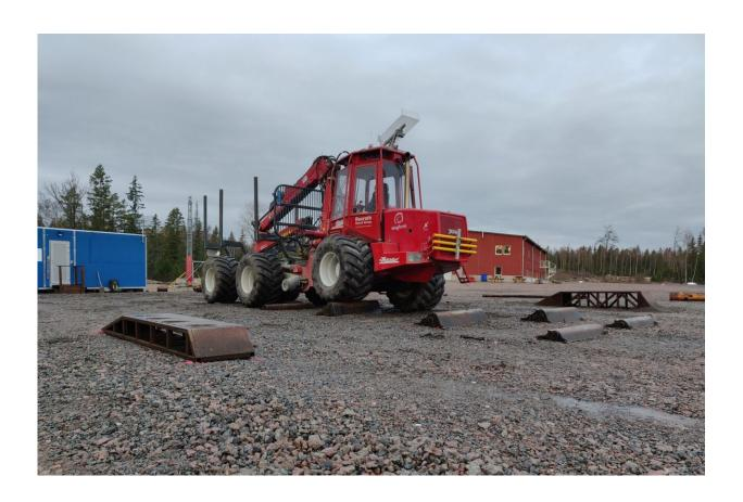
The Xt28 concept forwarder on an obstacle course at Skogforsk Troëdsson Forestry Teleoperation Lab. The forestry machine weighs 16 tonnes, has six wheels on hydraulically controlled pendulum arms and two steered centre joints. This gives the vehicle great freedom of movement in difficult terrain but makes the vehicle more challenging to control than a conventional forwarder. Credit: Viktor Wiberg
