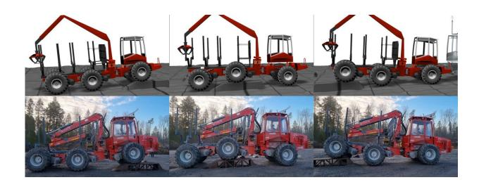
Comparison between the simulated and real forestry machine travelling over a high ramp, controlled by the same AI model (Policy C2). The model endeavours to maintain a steady speed toward the next target point with good and evenly distributed ground contact. It reacts to the power variations of the hydraulic system and laser data of the local environment. Credit: Viktor Wiberg
