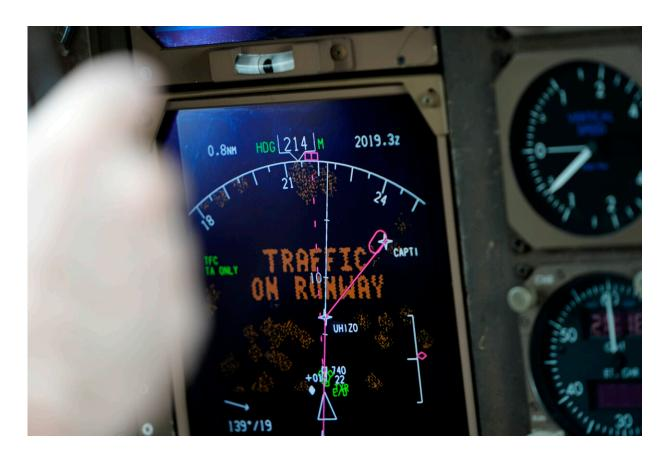
Honeywell test pilot Joe Duval pulls a Boeing 757 test aircraft out of a landing approach demonstrating runway hazard warning systems over the airport in Tyler, Texas, Tuesday, June 4, 2024. Credit: AP Photo/LM Otero
