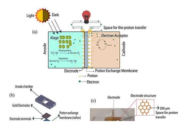
(a) Operating principle, (b) components of the  $\mu$ PSC, (c) photo image of the fabricated  $\mu$ PSC, (d) dimensions of the  $\mu$ PSC. Credit: *Energies* (2024). DOI: 10.3390/en17071749
