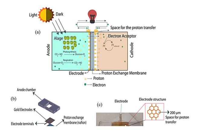
(a) Operating principle, (b) components of the  $\mu$ PSC, (c) photo image of the fabricated  $\mu$ PSC, (d) dimensions of the  $\mu$ PSC. Credit: *Energies* (2024). DOI: 10.3390/en17071749
