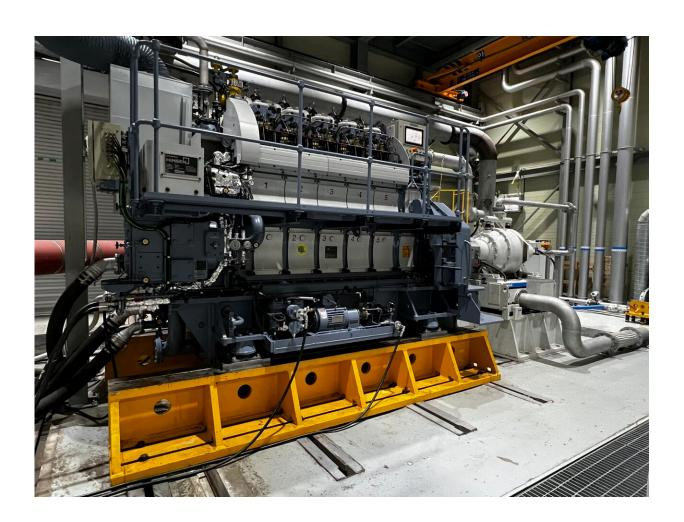
MW-class demonstration LNG-ammonia dual-fuel marine engine in KR TCC. Credit: Korea Institute of Machinery and Materials (KIMM)
