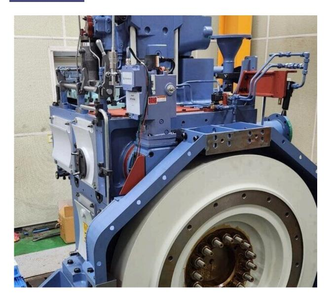
Large single-cylinder LNG-ammonia dual-fuel marine engine in KIMM. Credit: Korea Institute of Machinery and Materials (KIMM)
