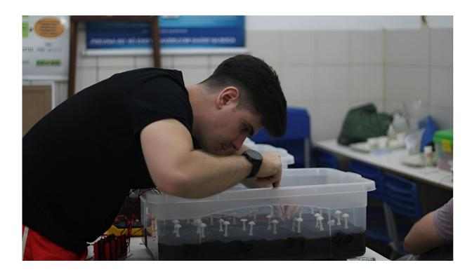
Checking on the bacteria-powered battery which harvests energy from microorganisms in the soil. Credit: Bactery
