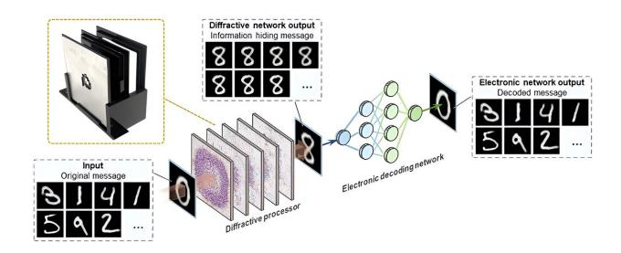
All-optical information hiding camera with electronic decoding. The diffractive processor all-optically conceals arbitrarily selected input images and transforms them into ordinary-looking "dummy" patterns that mislead human observers, whereas a following electronic decoder recovers the original image from these information hiding output messages. Credit: UCLA Engineering Institute for Technology Advancement
