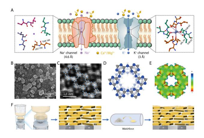
Bioinspired construction of PTIPCN composite membrane for LiMg separation. Credit: QIBEBT
