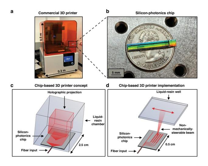
The chip-based 3D printer concept. Photographs showing a a typical commercial 3D printer with a photonic chip (outlined in black) for scale and b a fabricated and packaged photonic chip. c Conceptual diagram of the proposed chip-based 3D printer, showing a hologram formed by a chip within a resin chamber (not to scale). d Conceptual diagram of the proof-of-concept stereolithography-inspired
