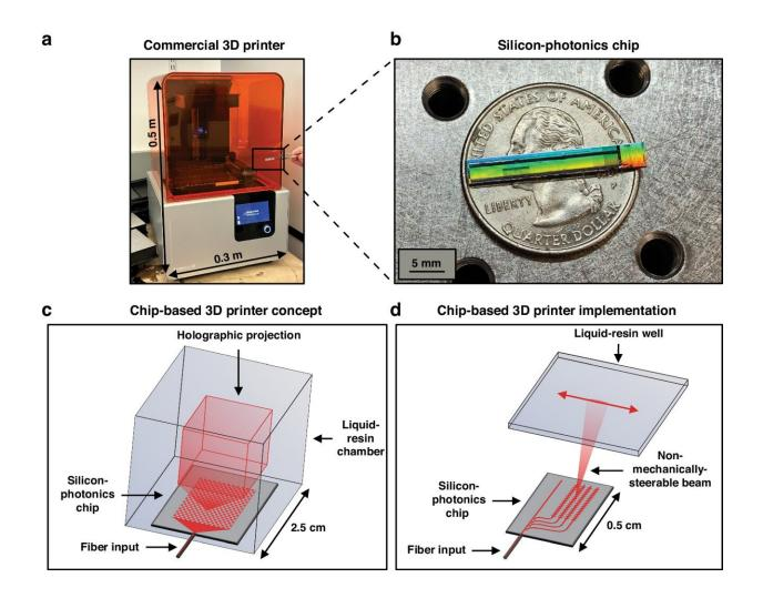
The chip-based 3D printer concept. Photographs showing a a typical commercial 3D printer with a photonic chip (outlined in black) for scale and b a fabricated and packaged photonic chip. c Conceptual diagram of the proposed chip-based 3D printer, showing a hologram formed by a chip within a resin chamber (not to scale). d Conceptual diagram of the proof-of-concept stereolithography-inspired
