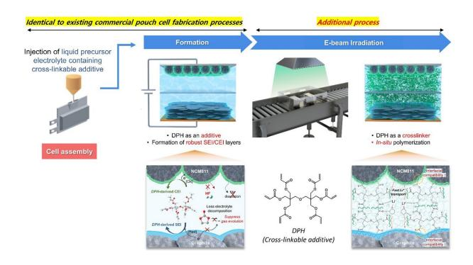
The manufacturing of pouch-type batteries with final gel electrolyte is accomplished by following the identical manufacturing process as conventional commercial pouch cells, including the formation and degassing steps, with the addition of an electron beam process. Credit: POSTECH
