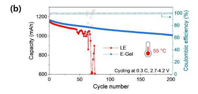
In high-temperature evaluations of a high-capacity pouch cell (1.2 Ah), it was confirmed that the gel electrolyte (E-Gel) operates reliably even after 200 cycles, compared to commercial liquid electrolyte (LE). Credit: POSTECH
