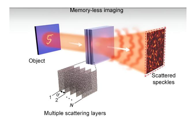
Schematic of scattering through multiple diffusers. Each diffuser can be modeled as a thin scattering layer, with N representing the number of diffusers and d representing the spacing between diffusers. Credit: *Science Advances* (2024). DOI: 10.1126/sciadv.adn2205
