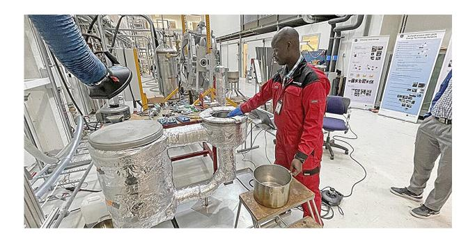
Jimmy Chaciga is a PhD candidate at Makerere University in Uganda. Here he is testing a solar cooker with heat storage at the Thermal Engineering Laboratories at NTNU. Credit: Ole Jørgen Nydal/NTNU
