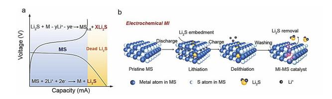
(a) Discharge and charge curves for MSs. (b) Illustration of electrochemical MI strategy. Credit: Science China Press
