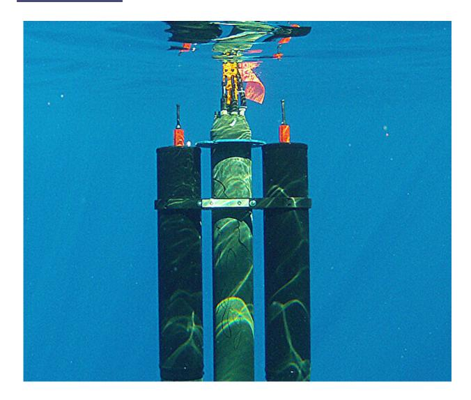
Two of Seatrec's SL1 modules are attached to a robotic float. The modules generate power from changes in volume undergone by phase-change materials as the float rises from colder deep water to warmer surface water. By adding a second module, the operator doubles the available energy. Credit: Seatrec
