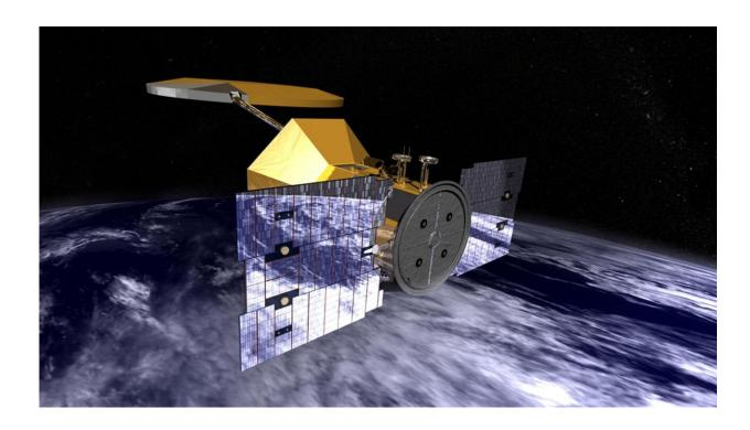
NASA's Aquarius instrument aboard the joint U.S. and Argentinian Satélite de Aplicaciones Científicas mapped the surface salinity of Earth's oceans between 2011 and 2014. To calibrate the instrument, a team from NASA's Jet Propulsion Laboratory, including project scientist Yi Chao, had to distribute robotic floats across oceans. The experience helped inspire Chao's invention of an inexhaustible power source for ocean floats and sensors. Credit: NASA
