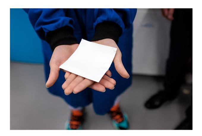
As solar light is visible and the thermal radiation emitting from buildings and pavement in an urban heat island is infrared, the UChicago Pritzker School of Molecular Engineering team had to engineer the fabric to exhibit two different sets of optical properties at the same time. Credit: John Zich / UChicago Pritzker School of Molecular Engineering
