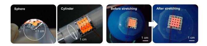
Photographs of stretchable OLEDs conformally attached to a sphere (left) and cylinder (right) with a radius of 1 cm and photographs of stretchable OLEDs conformally attached to a balloon before (left) and after (right) expansion. All of the operating OLEDs in photographs were driven with a constant current of 1 mA. Credit: *Nature Communications* (2024). DOI: 10.1038/s41467-024-48396-w
