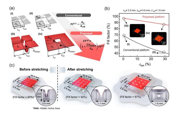
An overview of the proposed high FF stretchable OLED with a hidden active area (HAA). Credit: *Nature Communications* (2024). DOI: 10.1038/s41467-024-48396-w
