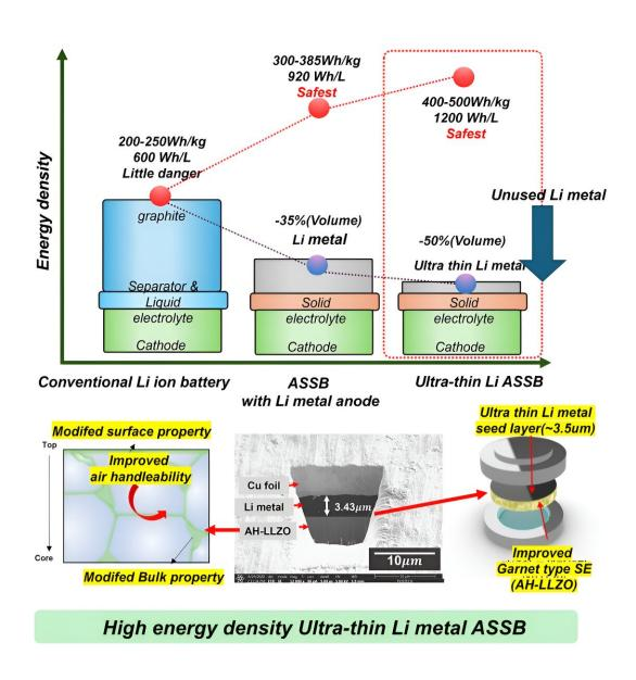
Enabling high energy density ultra-thin lithium metal solid-state batteries. Credit:
