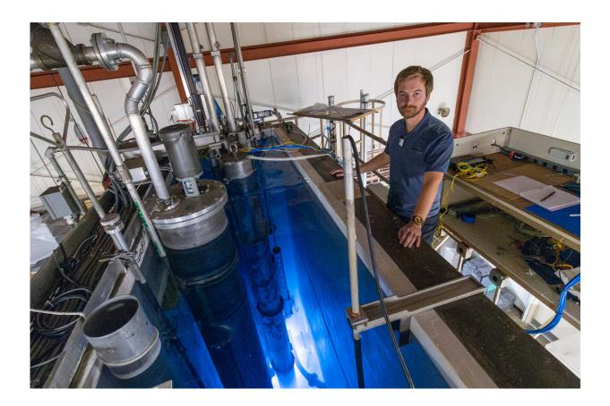
Kyle Reed led a team testing an ORNL-made, hardy new type of transistor in the reactor pool as it glows with radiation at The Ohio State University Nuclear Reactor laboratory. Credit: Michael Huson/The Ohio State University
