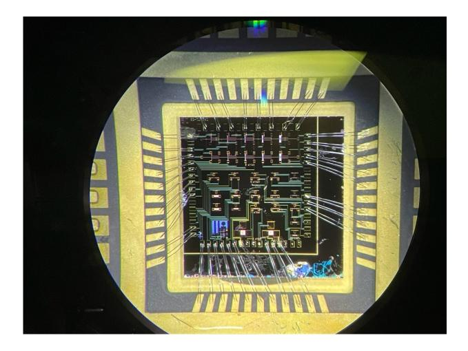
A wire-bonded die consisting of over 20 gallium nitride high-electron mobility transistors, seen here under a microscope, could be used in nuclear sensing equipment because of its high resistance to radiation. Credit: Kyle Reed/ORNL, U.S. Dept. of Energy
