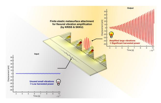
A conceptual illustration demonstrating the vibration amplification performance of the metamaterial developed by KRISS. The metamaterial can amplify typically discarded micro-vibrations by more than 45 times. Credit: Korea Research Institute of Standards and Science (KRISS)
