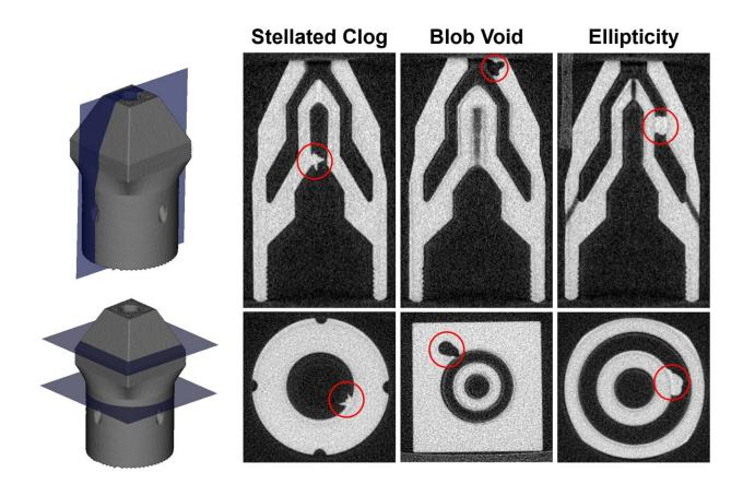
Longitudinal (top) and axial (middle) images of X-Ray CT data of parts with 6 internal defects: a spherical clog, a stellated shaped clog, a cone shaped void, a blob shaped void, an elliptical warp of the inner channel, and a nonconcentric center nozzle. Credit: The Grainger College of Engineering at the University of Illinois Urbana-Champaign
