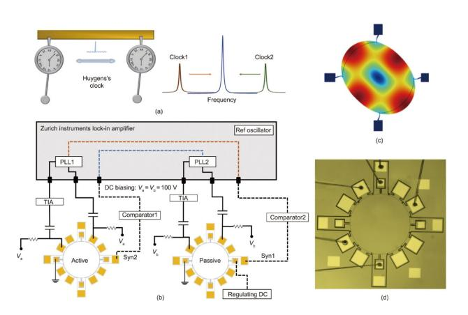
(a) Schematic of original Huygens's clock. (b) Structure of MEMS Huygens clock system. (c) Operating mode of MEMS resonator. (d) Image of microfabricated MEMS resonator. PLL: phase locked loop; TIA: transimpedance amplifier; Va: DC driving voltage of the active oscillator; Vb: DC driving voltage of the passive oscillator; Ref: reference. Credit: Xueyong Wei et al.
