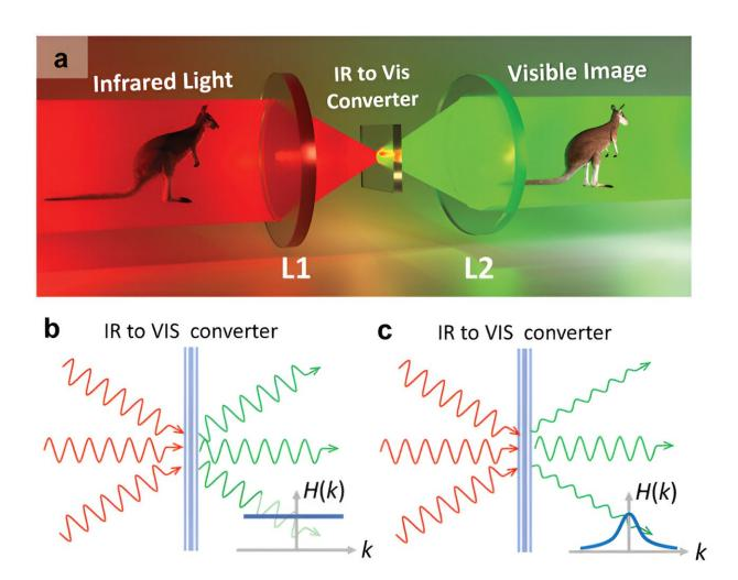
Infrared (IR) to visible (VIS) up-conversion for vision applications. a) Schematic of the nonlinear up-converter for infrared imaging, where infrared light illuminating an object and passing through a lens (L1) is coherently up-converted to visible light and captured by another lens (L2) to be finally observed on a conventional silicon-based camera. b) The ideal up-converter shall convert all
