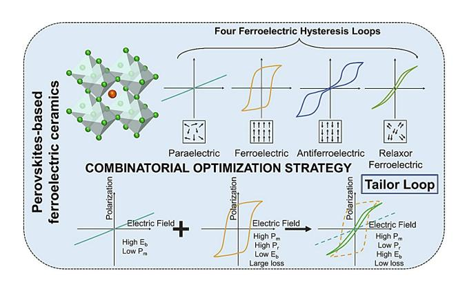
Dielectric materials be categorized into four types depending on the hysteresis loops they exhibit: paraelectric (PE), ferroelectric (FE), relaxor ferroelectric (RFE), and antiferroelectric (AFE). Tailor ferroelectric hysteresis loops via combining two dielectric materials, enhancing energy storage performance. Credit: Journal of Advanced Ceramics, Tsinghua University Press
