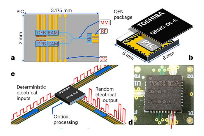
Implementation of a deployable OEC with integrated photonics. Credit: *Nature Electronics* (2024). DOI: 10.1038/s41928-024-01140-0
