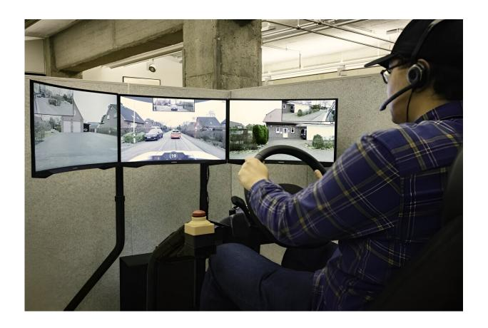
A Vay driver operates a vehicle remotely from a control center that features multiple video feeds. Tele-driving could offer many of the efficiencies that autonomous vehicles are expected to provide, according to research at U-M. Credit: Vay.
