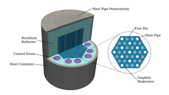
Basic layout of the Westinghouse eVinci microreactor design with an enlarged fuel flake. Credit: Price et al., 2024.
