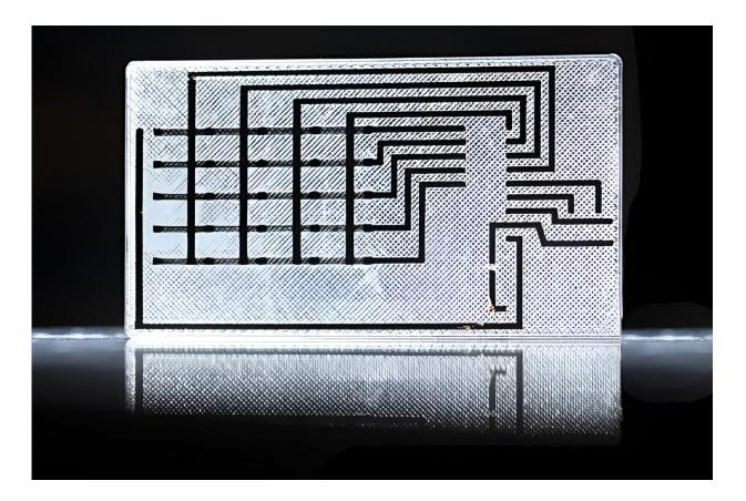
An example of electrodes printed inside of a plastic material. Credit: Sam O'Keefe
