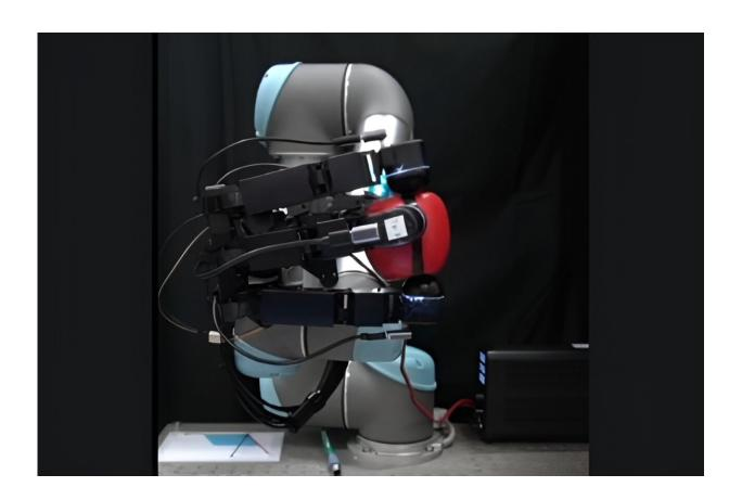
The team at the University of Bristol have created a four-fingered robotic hand with artificial tactile fingertips capable of rotating objects such as balls and toys in any direction and orientation Credit: University of Bristol
