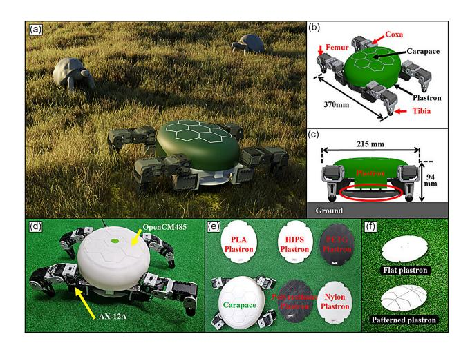
a) Tortoise-inspired belly-dragging robot. b) Schematic CAD design of tortoise-inspired belly-dragging robot. c) Side view of the robot. d) Tortoise-inspired belly-dragging robot with actuators (AX-12A) and extension board for TTL (OpenCM485). e) 3D-printed plastrons made of five different kinds of material. f) Flat and patterned plastron based on HIPS plastron. Credit: *Advanced Intelligent Systems* (2024). DOI: 10.1002/aisy.202300720
